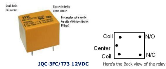
MAX. SWITCHING CURRENT:7A, 10A MAX. SWITCHING VOLTAGE:28V DC/ 250V AC DIELECTRIC STRENGTH VR.M.S: BETWEEN OPEN CONTACTS =750VAC; BETWEEN COIL AND CONTACTS =1000VAC; BETWEEN CONTACTS FORM =1000VAC; AMBIENT TEMPERATURE: -40-+85oC; OPERATION/RELEASE TIME:=10/8MS CONTACT CAPACITY: 10A 125V, 7A 250V
