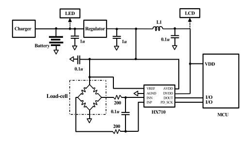
Fig. 1 Typical weigh scale application block diagram
