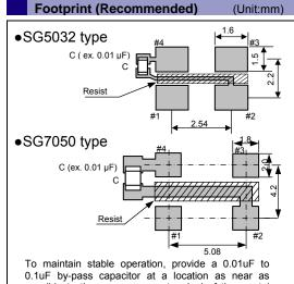
possible to the power source terminal of the crystal product (between Vcc - GND).
