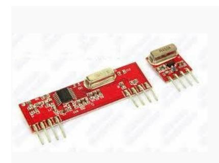
**Voltage** Supply voltage: 3 -12 V, Operation Voltage: 5 Volts
