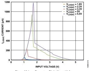
Figure 19. ILOGIC Current vs. Digital Input Voltage
