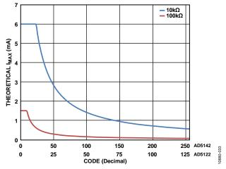
Figure 33. Theoretical Maximum Current vs. Code
