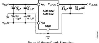
Figure 45. Power Supply Bypassing
