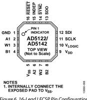
Figure 6. 16-Lead LFCSP Pin Configuration
