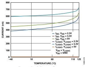
Figure 16. Supply Current vs. Temperature
