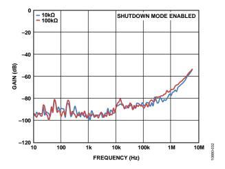
Figure 32. Shutdown Isolation vs. Frequency
