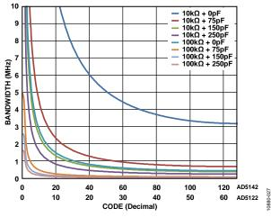
Figure 27. Maximum Bandwidth vs. Code vs. Net Capacitance
