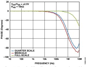
Figure 22. Normalized Phase Flatness vs. Frequency,  $R_{AB} = 10 k\Omega$
