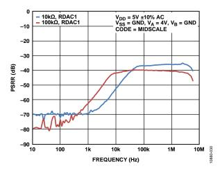
Figure 30. Power Supply Rejection Ratio (PSRR) vs. Frequency
