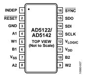
Figure 7. 16-Lead TSSOP, SPI Interface Pin Configuration
