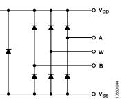
Figure 44. Maximum Terminal Voltages Set by V<sub>DD</sub> and V<sub>SS</sub>
