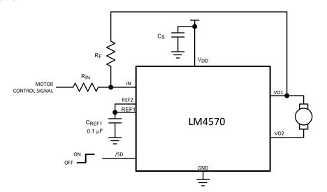
Figure 1. Typical Motor Driver Application Circuit
