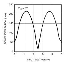
Figure 20. Power Dissipation vs. Input Voltage
