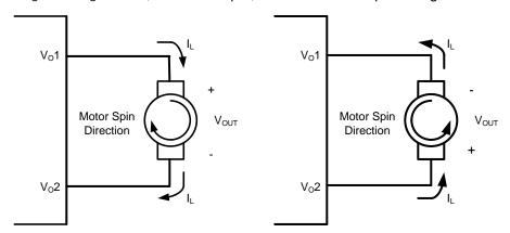
Figure 19. Voltage Polarity and Motor Direction
