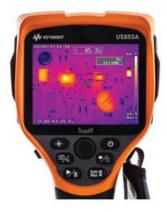
$\label{thm:condition} \textit{Figure 1. Detecting hotspot on a circuit board using Keysight U5850 series TruelR Thermal Imagers with image logging capability$
