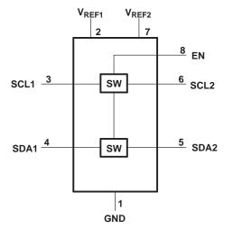
Figure 6. Block Diagram of PCA9306
