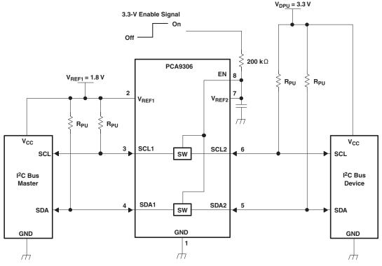
Figure 8. Typical Application Circuit (Switch Enable Control)
